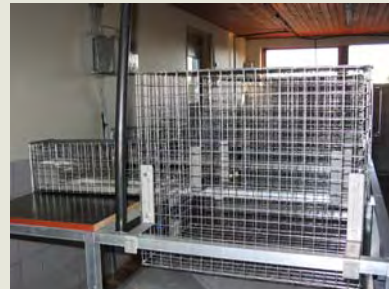
Digestibility cage, designed for measurement of feed intake, faeces and urine excretion
