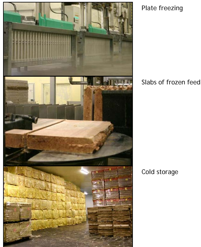
Figure 5 Feed production: plate freezing and storage
